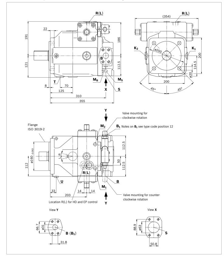
Main dimensions only for the basic unit, further dimensions are given in the relevant data sheets.
