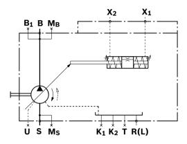
**Control system HS, HS5, with servo or proportional valve** (for further information, see data sheet 92076)
