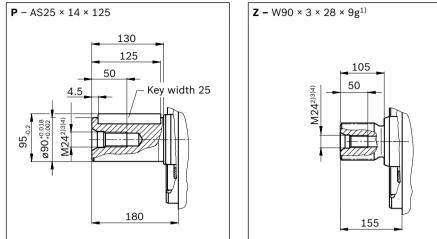
Splined shaft (DIN 5480)
