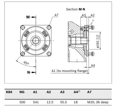
1) Mounting bolts and O-ring seal are included in the scope of delivery
