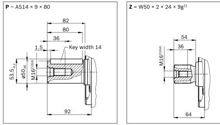
Splined shaft (DIN 5480)
