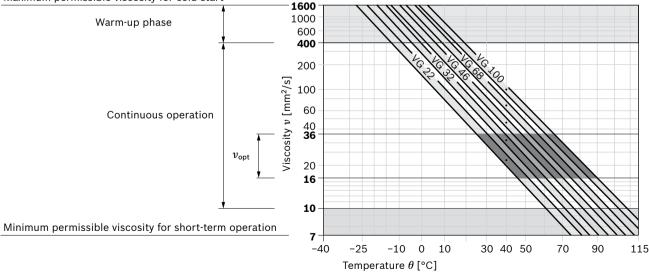
1) This corresponds, for example on VG 46, to a temperature range of +4 °C to +85 °C (see selection diagram)
