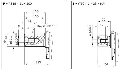
Splined shaft (DIN 5480)
